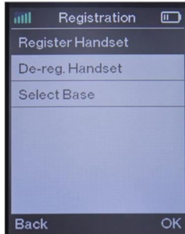
To register a handset to multiple base stations, press the **OK** navigation key, select **Settings > Registration > Register Handset** and repeat steps 2 through 5 above. Be sure to choose a base station that is not already selected or else it will overwrite the existing selection.
